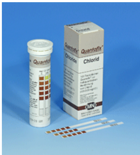
Figur 7.15 Strips for Quantab-analyse. (Foto: Multiconsult AS)
