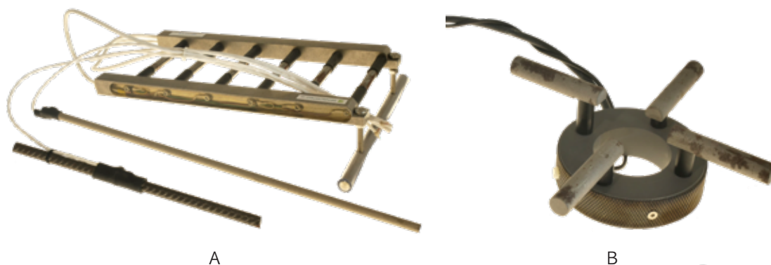
Figur E-2: Et utvalg sensorer for betong. (A) Anode-Ladder-System sensor, (B) CorroWatch sensor (Foto: Protector AS).
